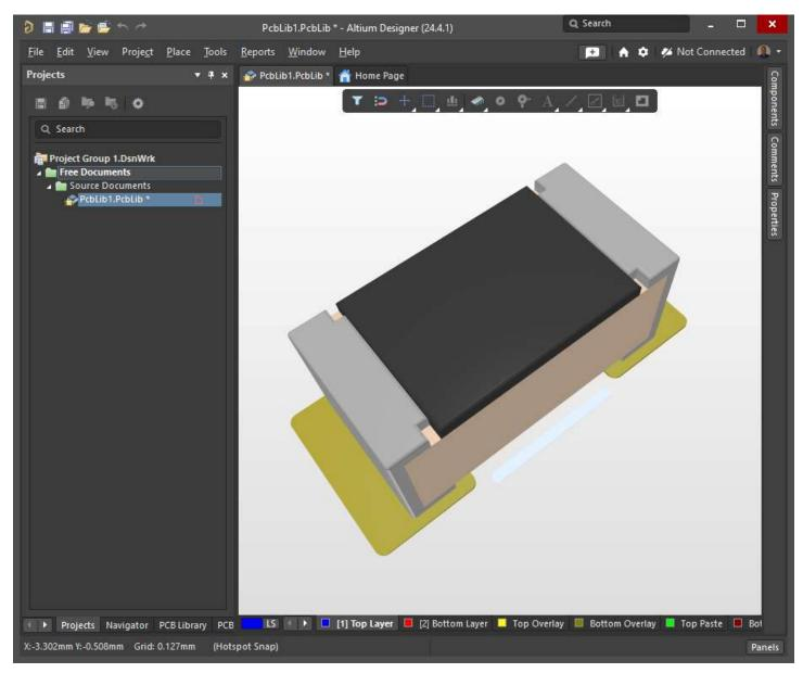
Use the "Shift + Middle Mouse Button" to rotate the 3D model.
